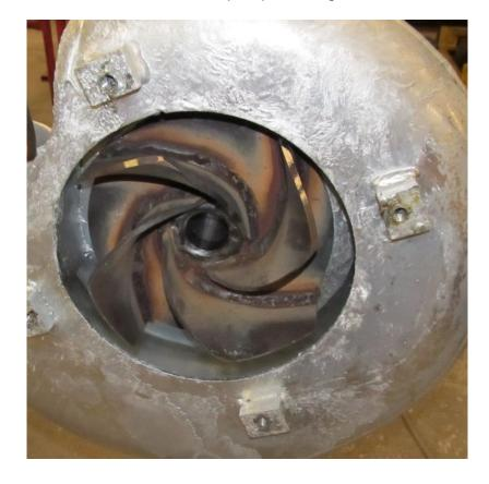
Pull the drive shaft and impeller out through the pump housing. As a result, the double joint and the bearing at the opposite will detach from the drive shaft.
