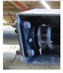
Take out the breaker bolt which secures the drive shaft to the double joint. Release the set screws on the bearing.
