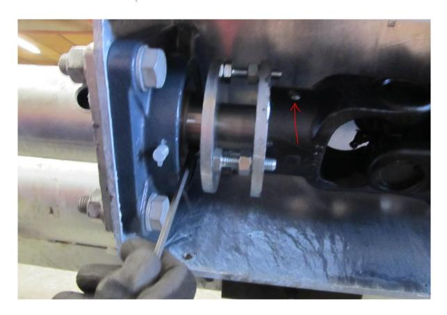
Release the cutter on the pump housing.
