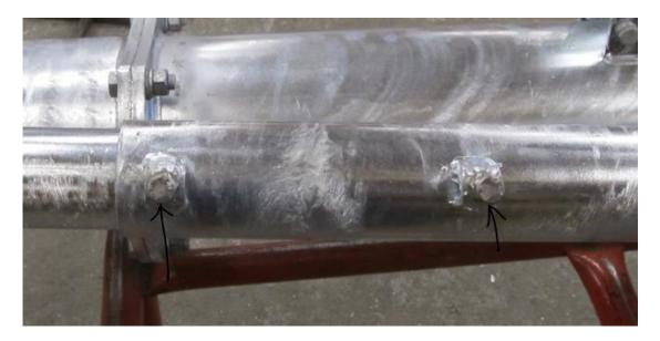
Release the cover tube where it is attached to the upper bearing. The bearing will also become loose.
